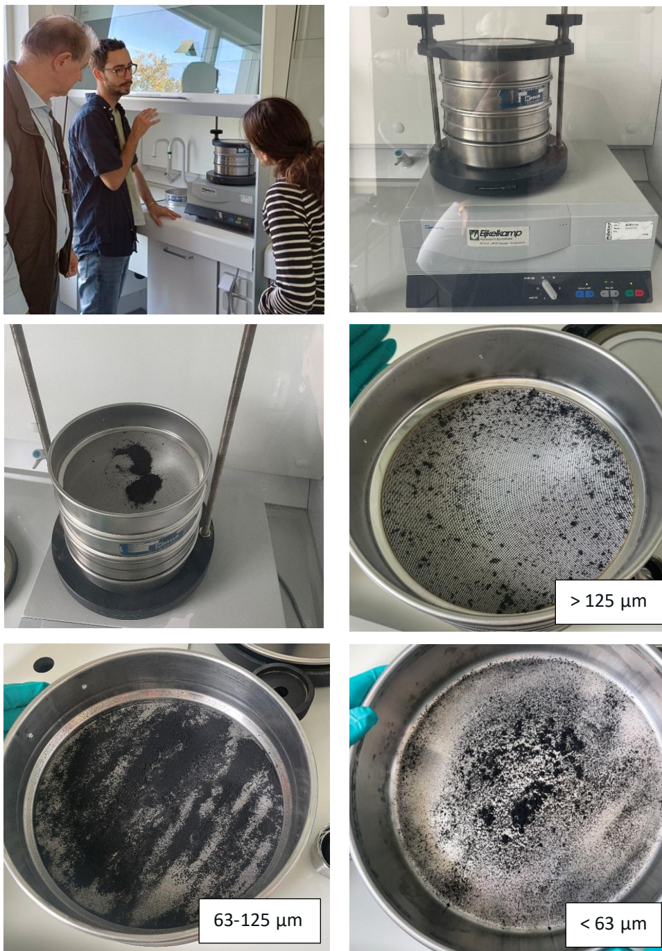
Figure 4: Sieving of cryo-milled UV-weathered biodegradable mulching film.
