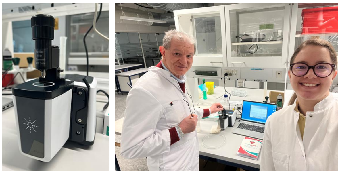
Figure 5: FTIR instrument (left) and FTIR analysis of plastic mulching films in progress (right).
