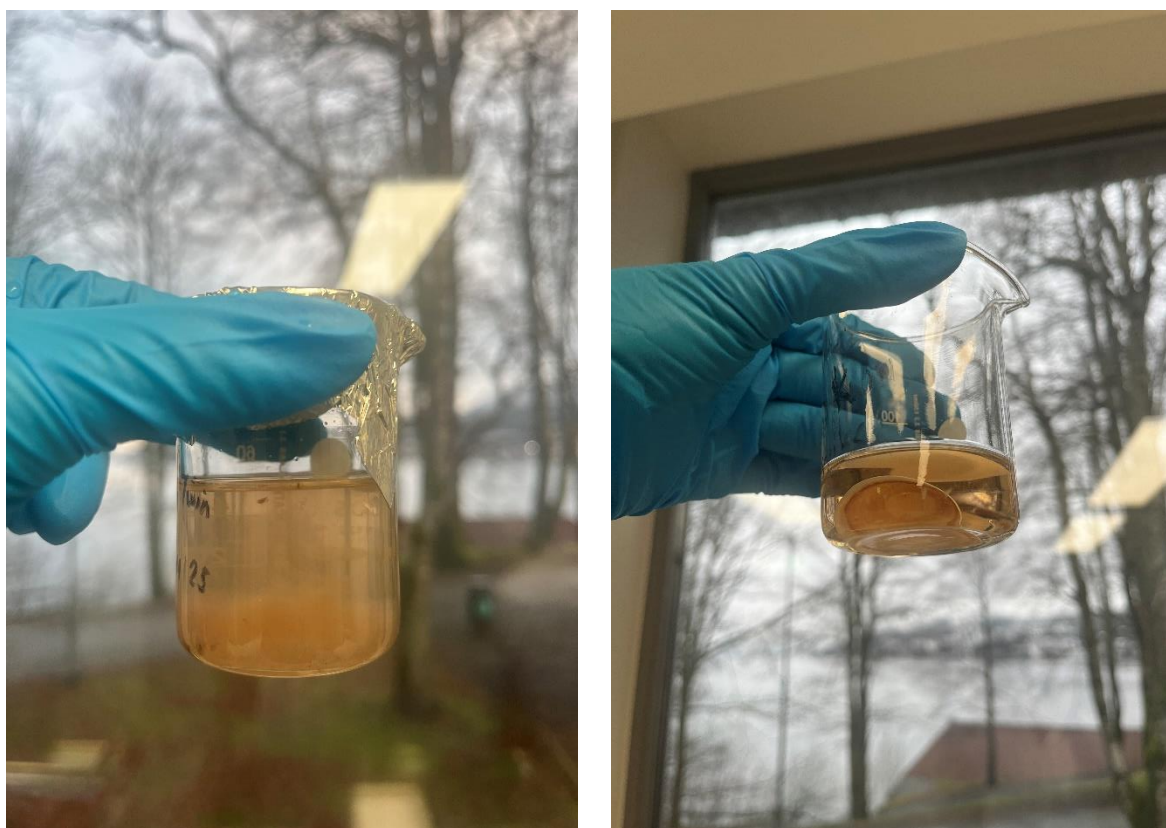
Figure 25. Step 1: Enzymatically digested sample (left) and Step 2: The 5 \mu\text{m} filter after filtration of the digest, suspended in 10% KOH (right).
