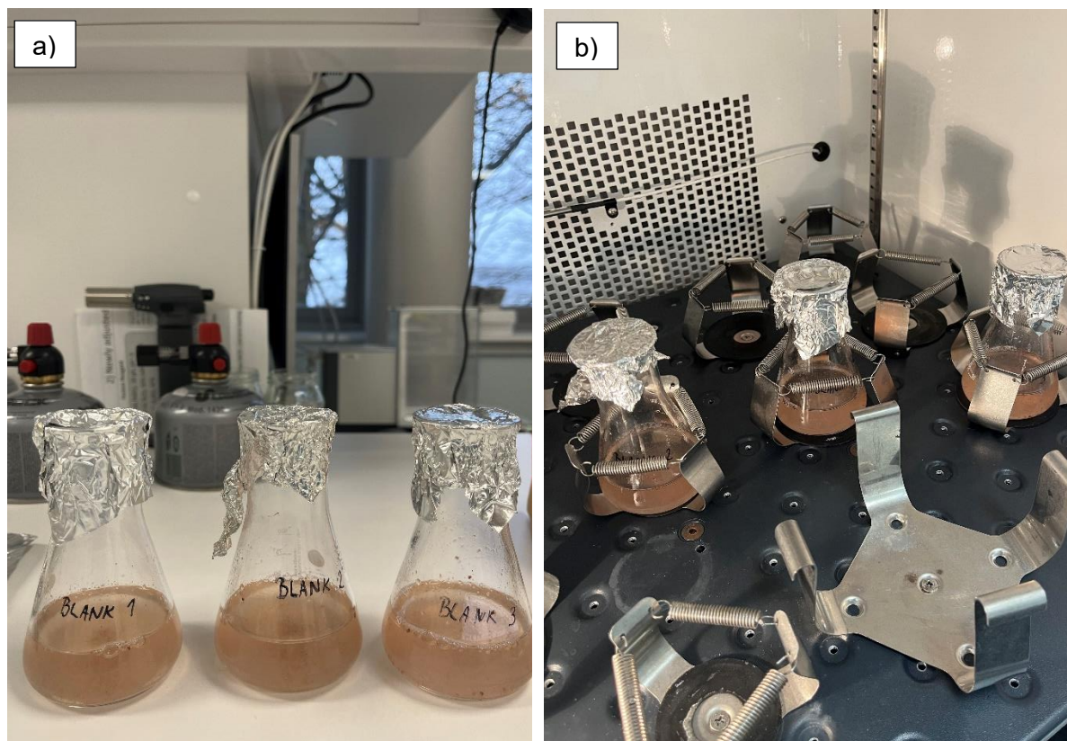
Figure 19. Initial upscaled sample preparation: a) samples after addition of citrate buffer and enzyme solution; b) samples placed in the incubator.
