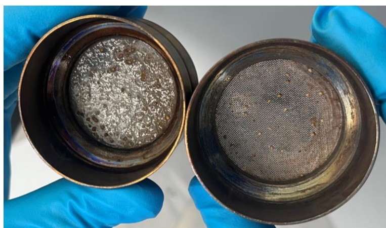
Figure 21. Stainless steel mesh filters following filtration of the strawberry digests, showing the 180 \mu\text{m} mesh (left) and 315 \mu\text{m} (right).
