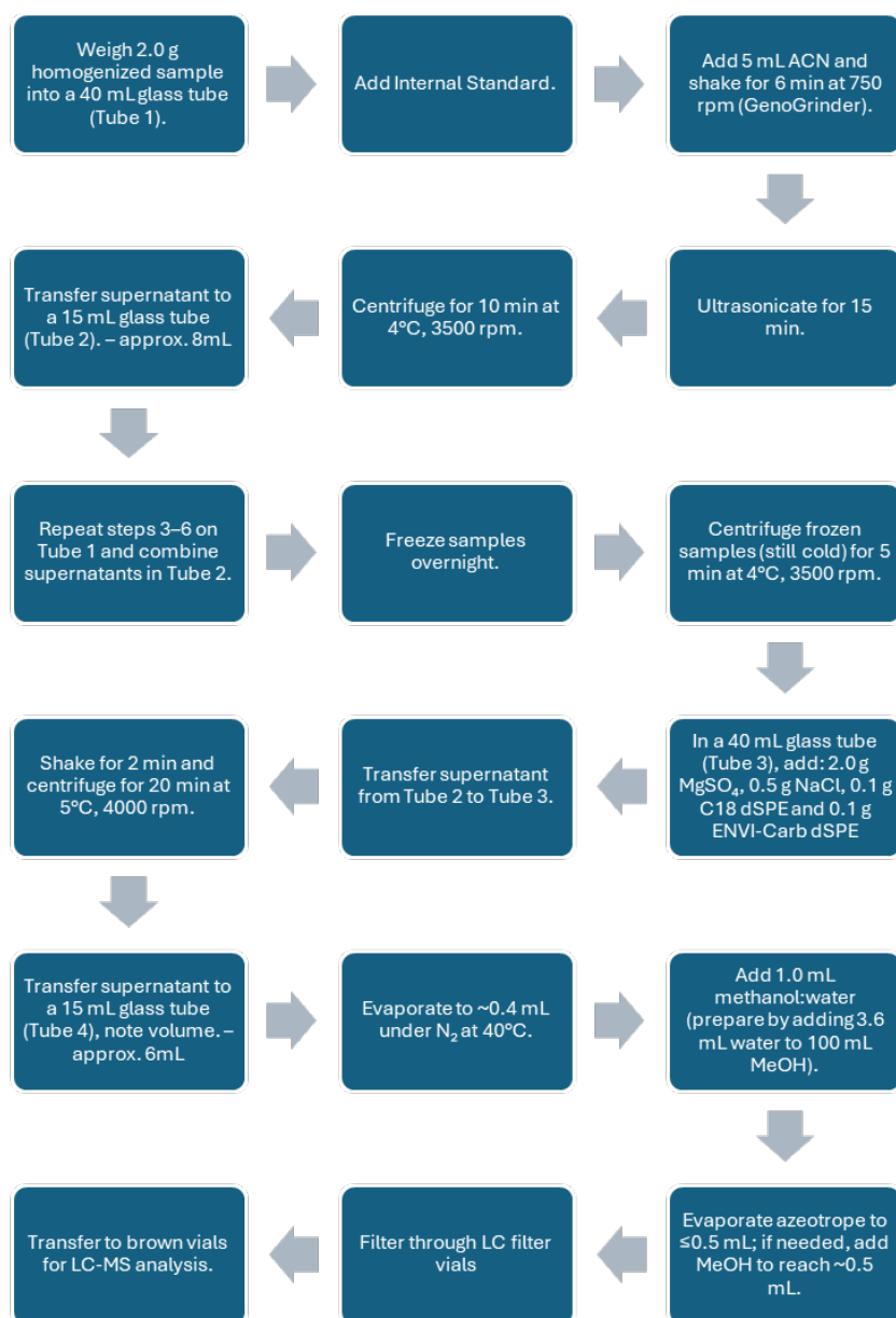
Figure 6. Steps for QuEChERS of strawberries
